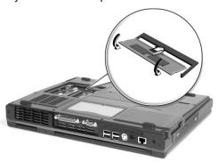
4 Replace the memory compartment door, and fasten the screw. The computer automatically detects the new module and reconfigures the memory.
